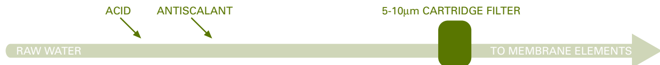
Figure 1. Simple pretreatment schematic when operating on typical deep well water.
